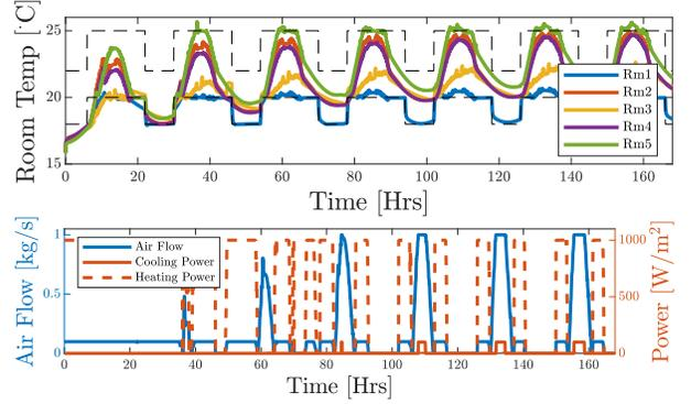
Fig. 2. FES controller for temperature regulation in a smart building. The comfort temperature (output) constraints are (approximately) satisfied throughout the simulations, while heating and cooling effort is minimized.
