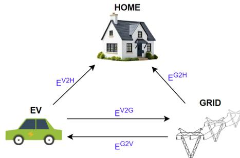
Fig. 1. Vehicle-home-grid interaction of the proposed algorithm. The arrows indicate the allowable energy flows for V2H, V2G, G2V and G2H.
