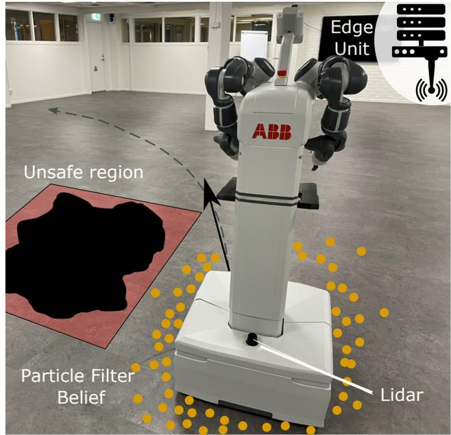
Fig. 1: A robot is navigating based on an offloaded particle filter localization, and needs to avoid the unsafe region based on the particle belief.
