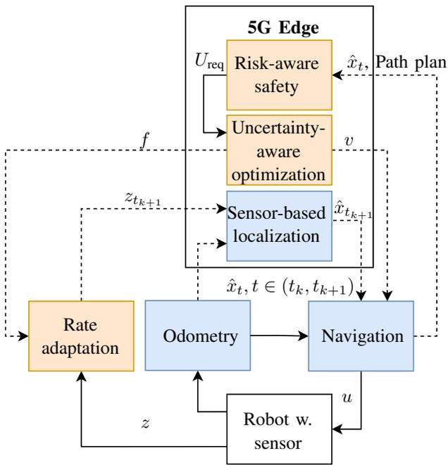
Fig. 2: The system architecture, with proposed components in yellow and existing functionality in blue.
