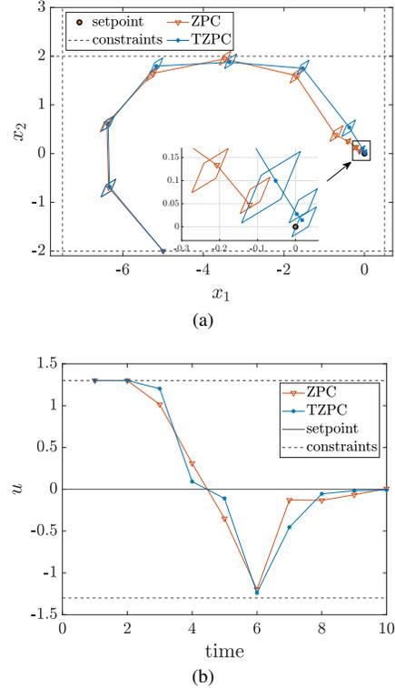
Fig. 1: Comparison between ZPC and TZPC. (a): The reachable sets for the closed-loop system. (b): Optimal control input.
