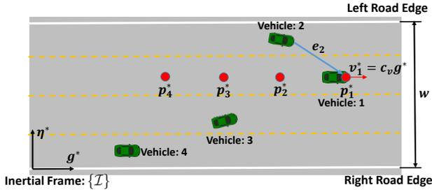
Fig. 1: Platoon formation scenario in a multi-lane highway segment at a certain time instance. The red dot indicates the desired position for each vehicle. The red arrow indicates the desired velocity for the platoon leader. The blue arrow between vehicle 2 and vehicle 1 indicates the relative position vector  $e_2$ .
